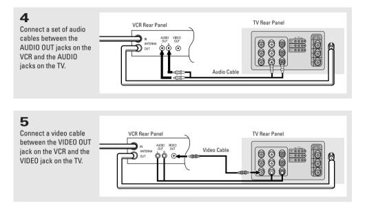
Follow the instructions in "Viewing an External Signal Source" to view your VCR tape. Note: This figure shows the Standard connector-jack panel. The actual configuration for your TV may be different.
