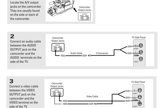
The audio-video cables shown here are usually included with a Camcorder. (If not, check your local electronics store.) If your camcorder is stereo, you need to connect a set of two cables.
