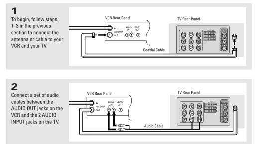
Make sure the jacks you are using are underneath the number "2."
