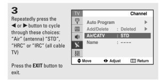
Note: STD, HRC and IRC identify various types of cable TV systems. Contact your local cable company to identify the type of cable system that exists in your particular area.
